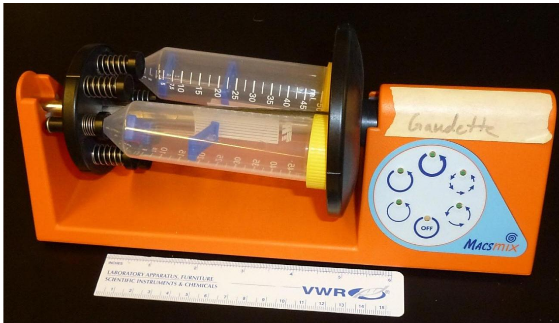
Figure 29: Seeding bioreactor assemblies in 50 mL conical tubes mounted on a tube rotator.
