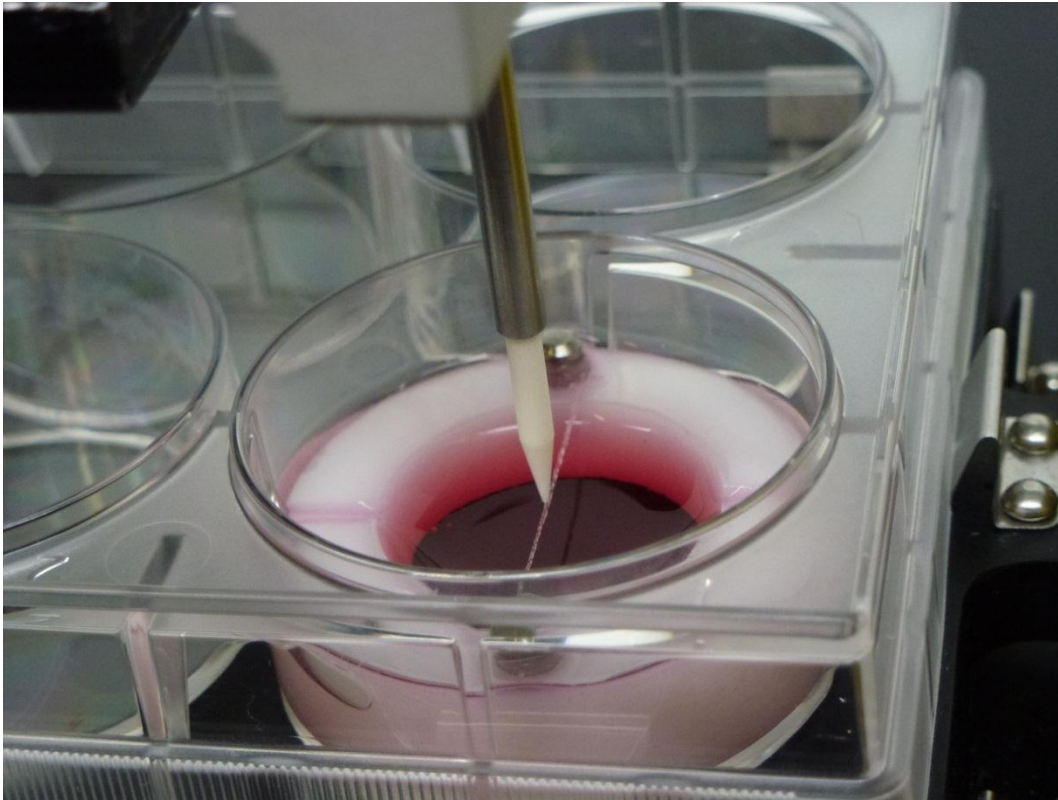
Figure 33: Cell printer's tip positioned over the thread bundle ready to begin dispensing hMSC-suspension
